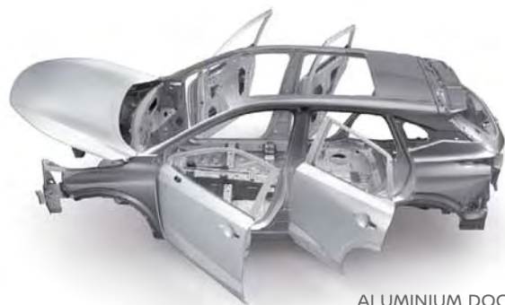
ALUMINIUM DOOR PANELS AND BONNET Lighter aluminium panels in both the door and bonnet help to reduce vehicle weight leading to a reduction in CO 2 emissions whilst driving.
